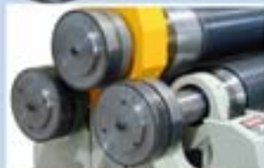
Extended Shafts are standard (up to model 25/7) for use with optional profile rolling dies.
