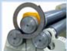
Optional Profile Rolling Dies Shown Mounted on Standard Extended Shafts will roll Flats, T and L shapes. Tube & Pipe Dies Available
